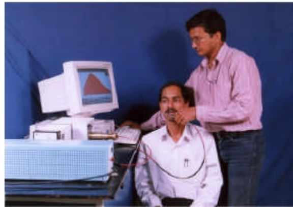
Nitrogen-laser-based system for oral cancer diagnosis developed at Center for Advanced Technology, Indore, India © with courtesy of CAT, Indore, India
